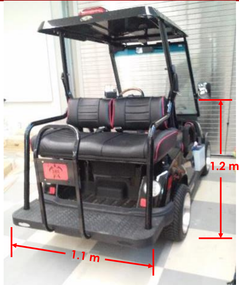
Figure 2. Photo of the back of the golf cart with recessed region under the rear seat.
