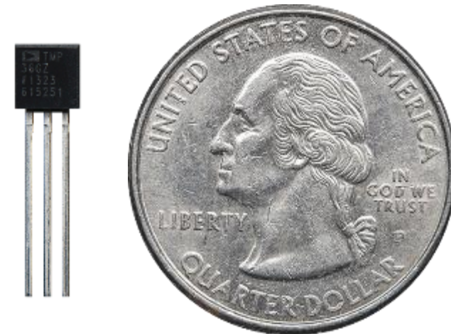
Figure 12. TMP Sensor. Quarter for scale [6]
